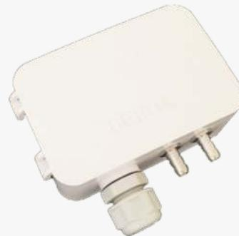
LFM108 differential pressure transmitter detect differential pressure or gauge pressure then convert this pressure difference to a proportional analogue output signal. Two output version are offered: Voltage output of 0~10VDC, and a current output 4-20mA. LFM108 differential pressure transmitter ranges from 0~±50Pa to 0~±10000Pa.
