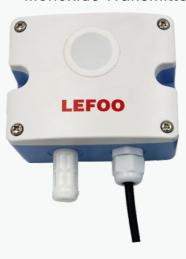
LFG series Carbon Monoxide Transmitters use electrochemical principles to detect carbon monoxide in the air, with good selectivity and stability Carbon Monoxide and Oxygen undergo redox reaction on the working electrode and the counter electrode, releasing charges to form current. The concentration of Carbon Monoxide can be determined by measuring the volume of the current. It applicable for precision gas
