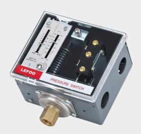
LF56 series pressure switches are mainly used to control pressure of boiler or water tower regulating system. When the system pressure exceed the setting point, the switch will cut off the circuit for protection. With SPDT contact arrangement, LF56 switch can detect the pressure change and shift the internal status accordingly to control the on/off of external circuits, which is available for the pressure control, limit and alarm of non-hazardous liquid, gas and steam.
