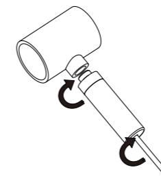
Wire and sensor rotate simultaneously to prevent wire breakage
