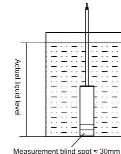
Attention should be paid to keeping the wiring harness perpendicular to the ground during the investment type liquid level
