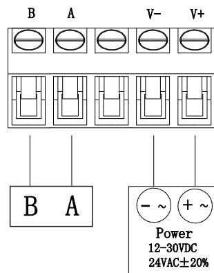
RS485 output wiring diagram
