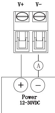
Current outputWiring diagram
