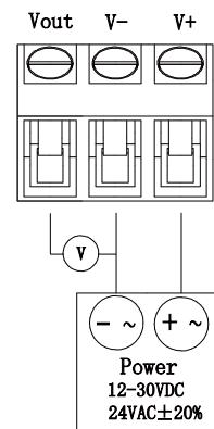
Voltage output wiring diagram
