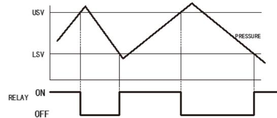
The relay automatically loads ON/OFF is according to the set starting pressure (LSV) and stopping pressure (USV).
